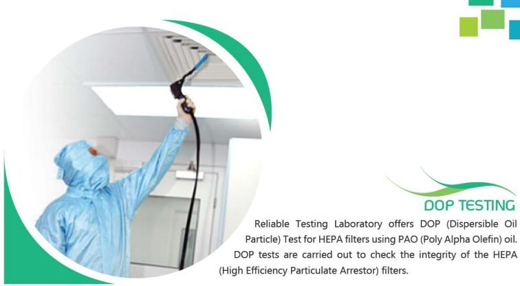
Reliable Testing Laboratory offers both onsite and offsite tests for your HEPA filtered equipment. Our technicians use state of the art equipment and are well trained, certified and experienced. DOP testing is done using the safest procedures and conform to international standards. Reliable Testing Laboratory can also test for Clean Rooms.
